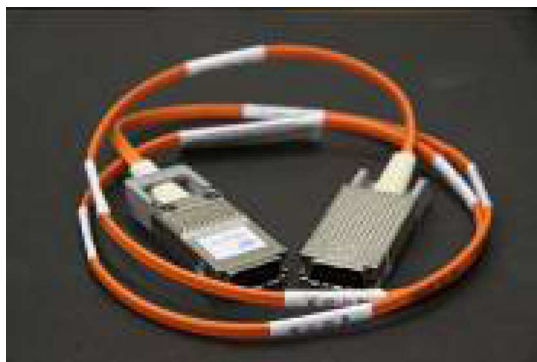
Fig. 12. Example of an active optical cable.
